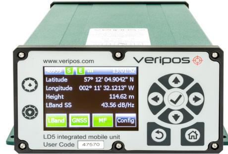
The LD5 Integrated Mobile Unit on-board colour display.
